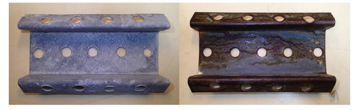
**Figure 6:** Results of accelerated corrosion testing (in the absence of chlorides) of batch galvanized sample (left) and ZM coated steel (right) after 10 cycles.
