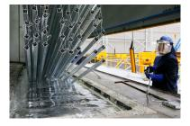
Post-galvanized EN ISO 1461 is applied after fabrication of steel conponents to ensure complete coverage of the coating.
