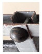
Cut edge protection for steel thickness greater than 2mm, where the cathodic effect reduces due to the reduced coating thickness, is especially questionable if the environment is not aggressive enough. Users of ZM coated steels have reported that red rust can still be seen after 25 months on 'self-healed' cut edges on parts situated in rural environments.
