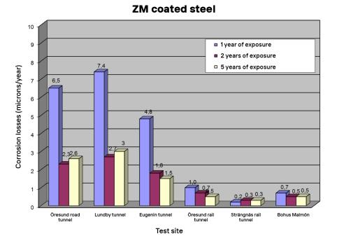
These tests showed no significant difference in the corrosion rate of zinc (galvanized) and ZM-coated steels. The expected coating performance would therefore be determined by the coating thickness as shown in Table 2.
