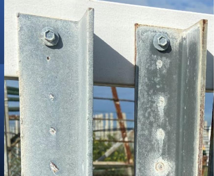
4 mm steel & HDG @ 100 microns VS 5 mm steel & Magnelis @ 21 microns
