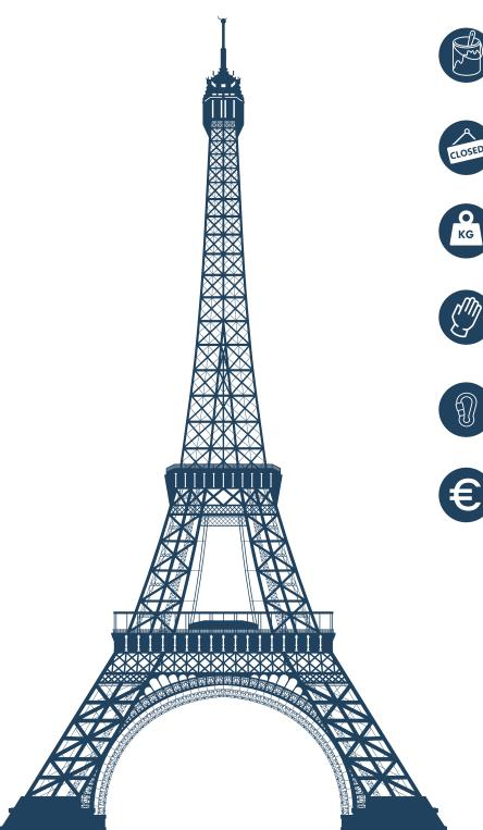
Each repaint applies 60 tonnes of paint and 15-20 tonnes of paint are eroded between each repaint
