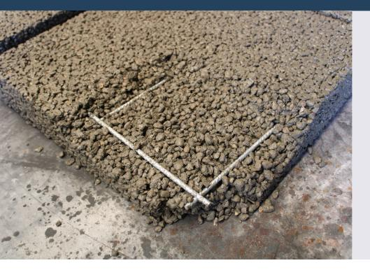
Galvanized steel reinforcement in concrete products and structures can provide a range of benefits. In aggressive environments, the need for increased concrete cover can be avoided. When lighter thinner concrete designs are required, galvanized steel reinforcement will protect against carbonation when concrete cover has been reduced.
